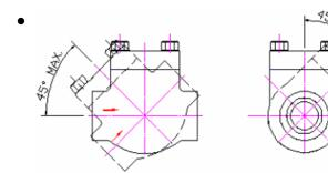
For vertical installation of the check valve, the flow must be in an upward direction so the disc seats when flow is reduced. The upstream pressure must exceed the cracking and downstream back pressure or else the valve may not open properly. Low flows can cause disc chatter, wear of seat and disc, and erosion.
